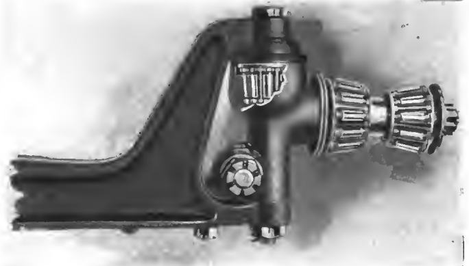
Front Axle with Timken Roller Bearing Knuckles.
